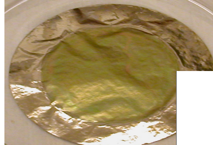
Showing 9.71 mg of ^{239}\text{Pu} on 3 \mu\text{m} Ti foil
